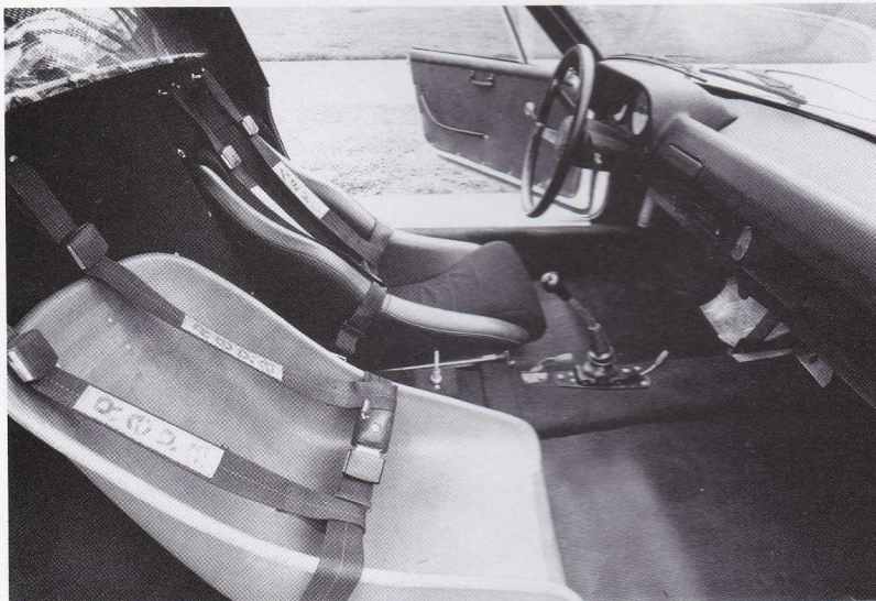
Porsche stripped clean the already spartan 914 interior, replacing the standard seating arrangement with a racing bucket for the driver and thin fiberglass shell for the "theoretical" passenger.
